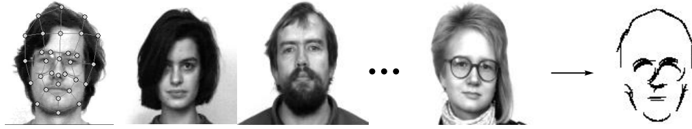
Figure 7: Left: 4 of 30 different training images. 31 landmarks are chosen for every face as shown in the leftmost image. Right: This is the learned representation for the object class “face”. There are some redundancies, e.g., in the area of the eyes and nose. The fact that there is only the left edge of the nose represented whereas the right is not, may derive from the fact that the illumination does not vary randomly in the training images. Note that irregularities such as glasses or a beard are not represented in the result.
