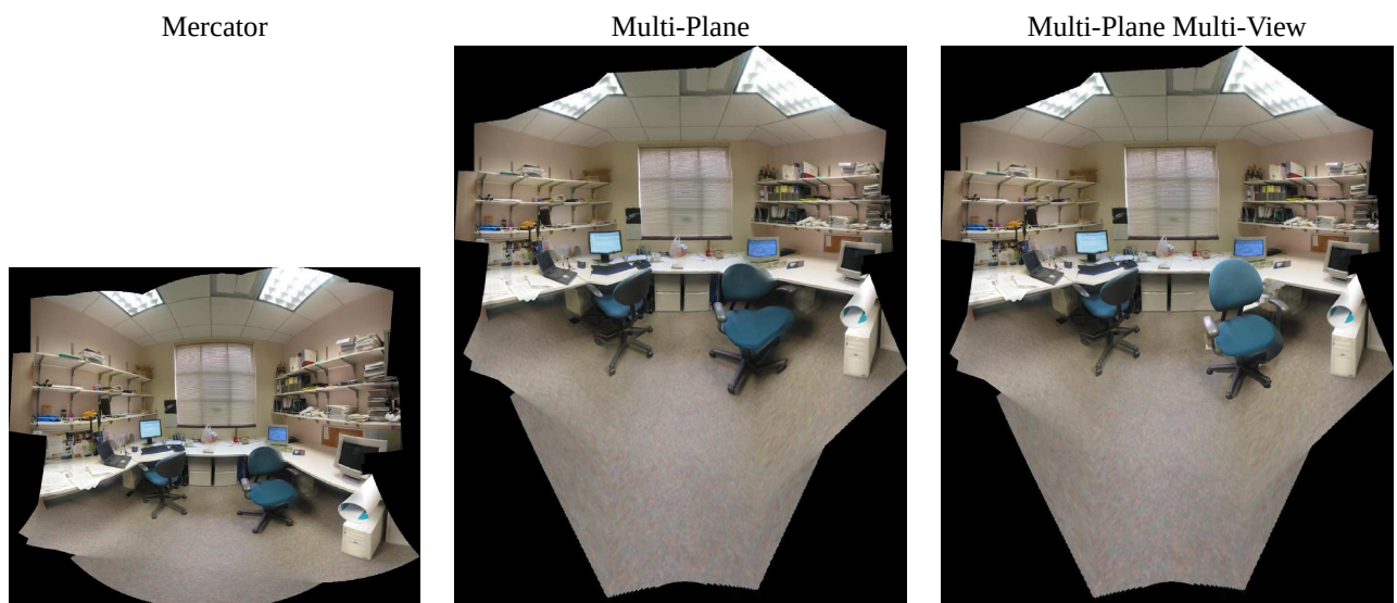
Figure 4: Multi-Plane Multi-View. The multi-plane projection rectified the background but the chair on the right got distorted. Using the Multi-View approach the chair is undistorted.
