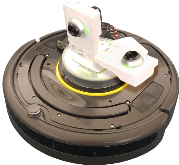
Fig. 10. Prototype configuration based on a vacuum cleaning robot.
