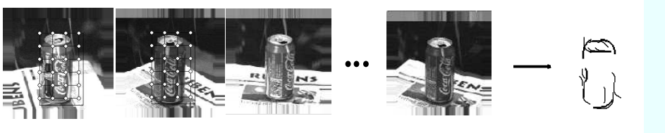
Figure 21: Automatic generation of ground truth for cans. i-iv: Rotated Cans on a rotating table with varying illumination (note the shadow of the can). i,ii: Rotated cans with rectangular grid. v) Learned Representation.
